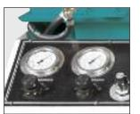
Hydraulic pressure gauges are mounted in the control panel. This lets the operator to easily adjust the blade cutting pressure and on models equipped with a hydraulic vise will let the operator adjust hydraulic vise grip pressure.
